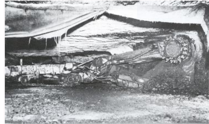
Early continuous miner in action. WVU
